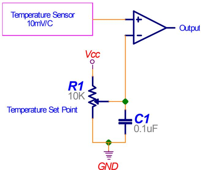
This is an example of a thermostat circuit. The temp sensor puts out 10mV/C (the [LM35](#) for example). The pot (short for potentiometer) lets the user dial in desired temperature. The capacitor helps to short any high frequency noise on the set point voltage to ground. Note: The cap isn't needed but it's a good idea to have it.
