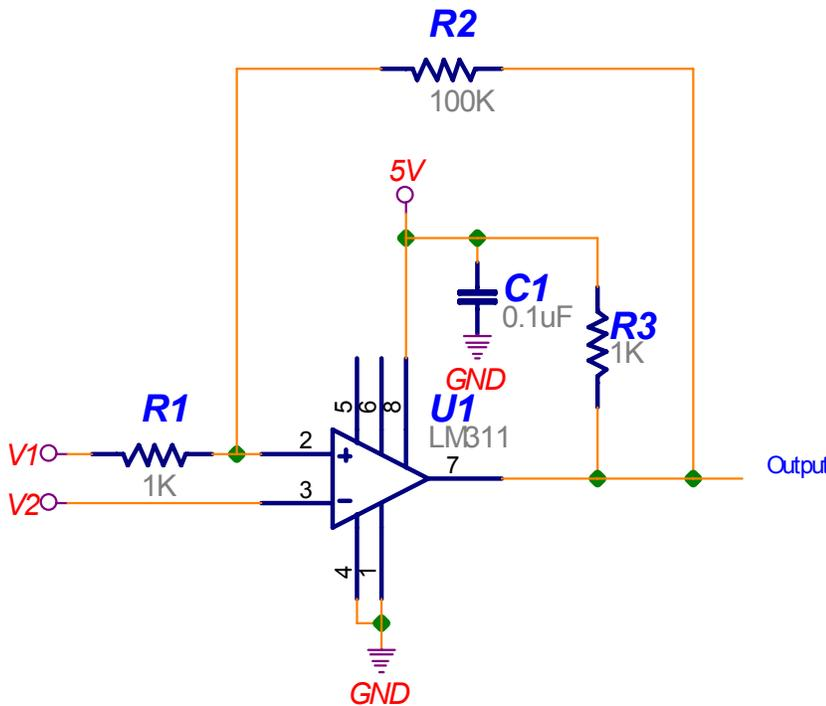
This circuit will compare two voltages,  $V_1$  &  $V_2$ , and will add a little hysteresis so that the output won't oscillate when  $V_1 = V_2$ . Note: Since the comparator is powered off a 0-5V supply the two input voltages should be between 0 & 5V.
