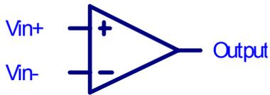
A comparator compares the voltages at the + and – inputs. If the + input is at a higher voltage than the – input the comparator output will be high. If the – input is at a higher voltage than the + input the comparator output will be low.
