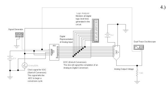
Load the **EWB** circuit file for the ADC/DAC system. Energize the file as supplied while monitoring the 'scope display. You stop can analysis after two cycles of the input. The input is a sinusoidal wave with a frequency of 1kHz. Compare the output to the input.
