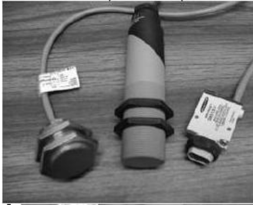
Figure 3-20 Inductive, Capacitive and Optical Proximity Switches
