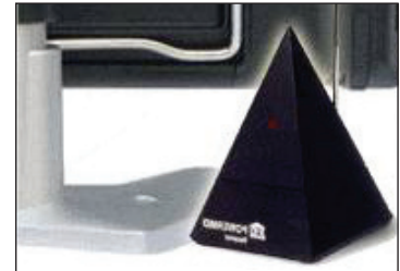
Figure 25. A RF TV remote can cause interference.
