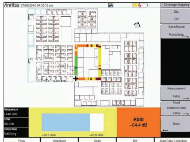
Figure 23. Plotting signal strength to find an interference source.
