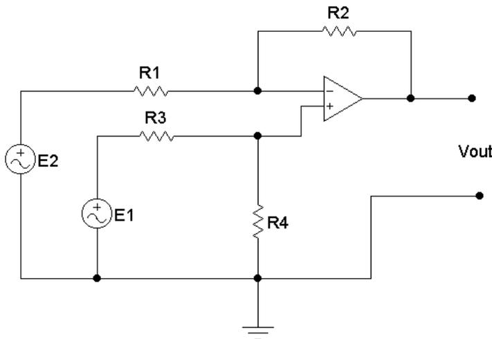
The differential-mode gain,  $A_{DM}$ , is the circuit gain measured with respect to the difference in potential between  $E_1$  and  $E_2$ .
