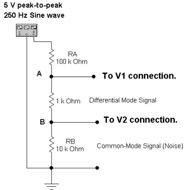
Once you have made the connections to your I.A., measure the output voltage of the I.A. using the oscilloscope. What do you observe?
