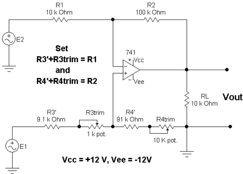
Calculate the expected  $A_{DM}$  for this circuit.  $A_{DM} =$  \_\_\_\_\_
