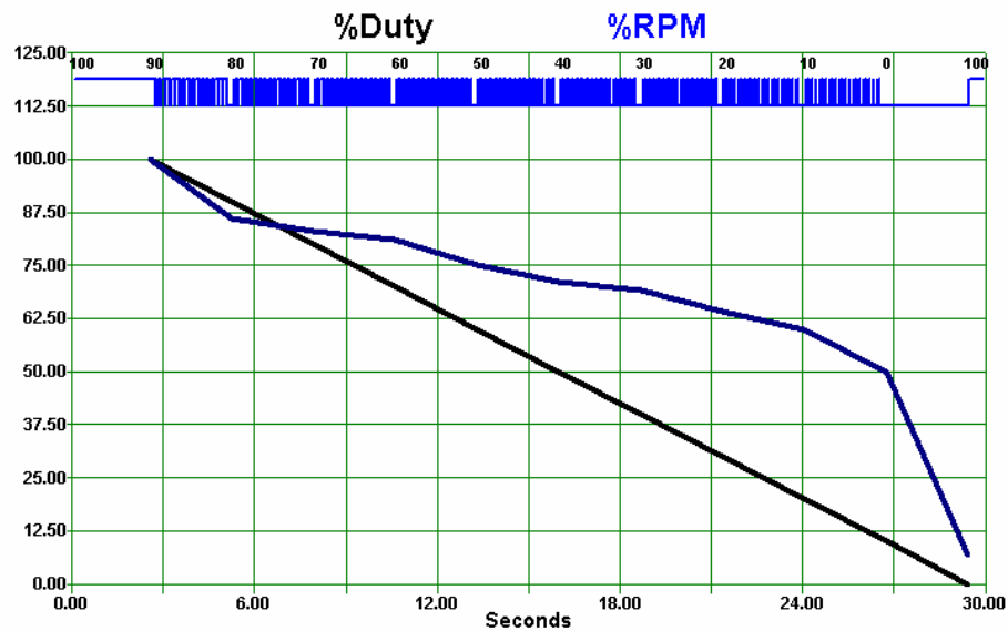
Figure 5-7 PWM Test with Manual Drive
