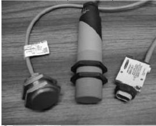
Figure 3-20 Inductive, Capacitive and Optical Proximity Switches
