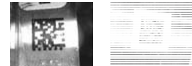
Diffuse dome lighting Reflective & curved surface DPM reading
