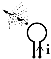
Loop = "transmitting" antenna
